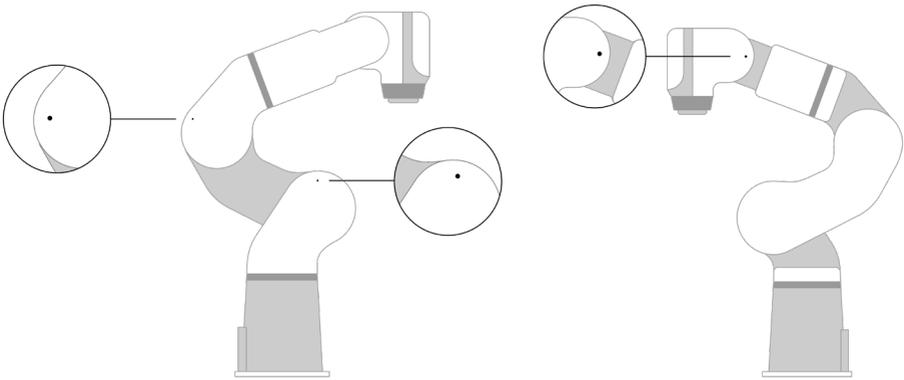
Diagram of brake release pin hole locations
