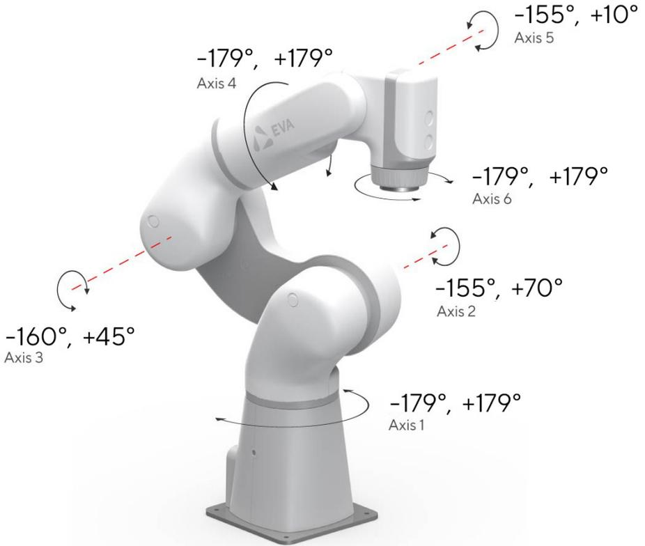
*NOTE: Axes 1, 4 and 6 have no mechanical limits (software only). The software limits are not safety-rated. The mechanical limits on axes 2, 3 and 5 are non-adjustable.*
